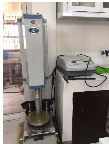
Fig. 5. Digital Compactor Machine
