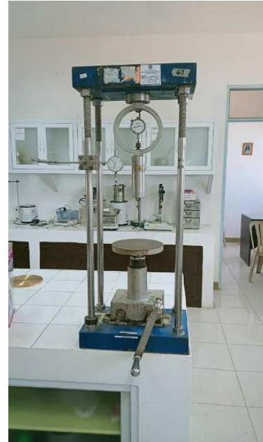
Fig. 4. California Bearing Ratio Machine
